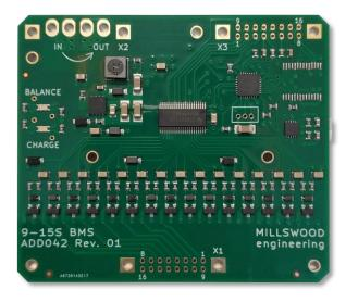
Figure 1 – 15S Battery Cell Monitor & Balancer
